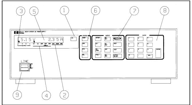
Figure 3-1. HP 6624A Front Panel
